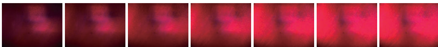
Change in color observed during the curing process
